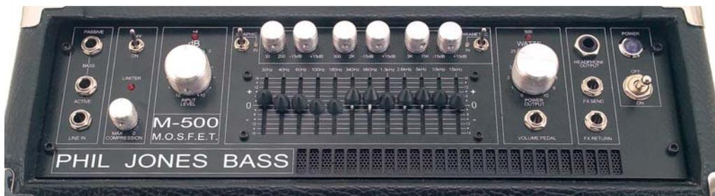
The M-500's front-panel features include a jack for an optional external volume pedal and an effect loop.
