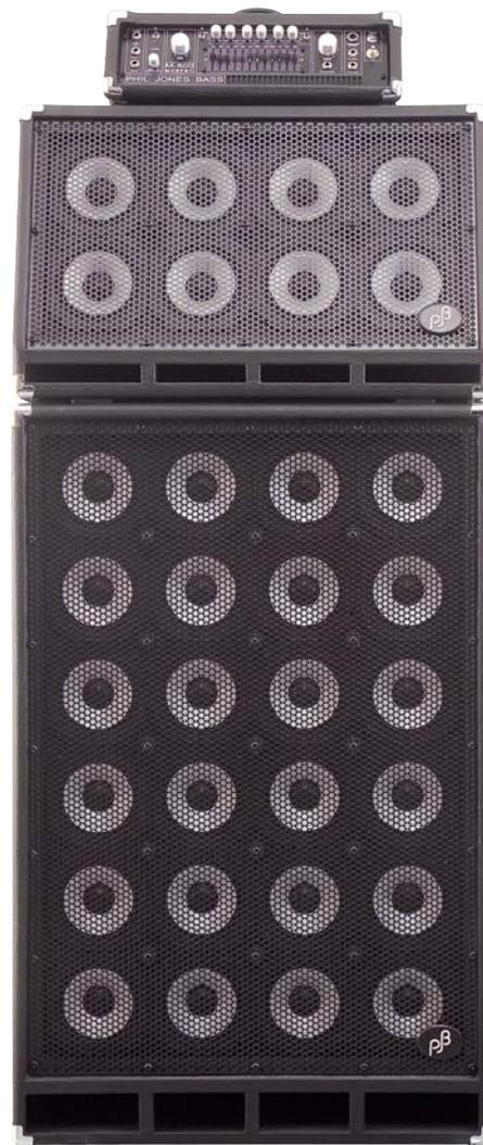
a 2x10 cabinet. But opposed to the two voice-coil "motors" of a 2x10 cabinet, the eight voice-coil equipped PJB cab has more motor driving the equivalent surface area. The result? Speed, resistance to dynamics-squashing compression, high power handling, and phenomenally loud output. The downsides? All those speakers, and the box to fit them in, are no-joke heavy.
