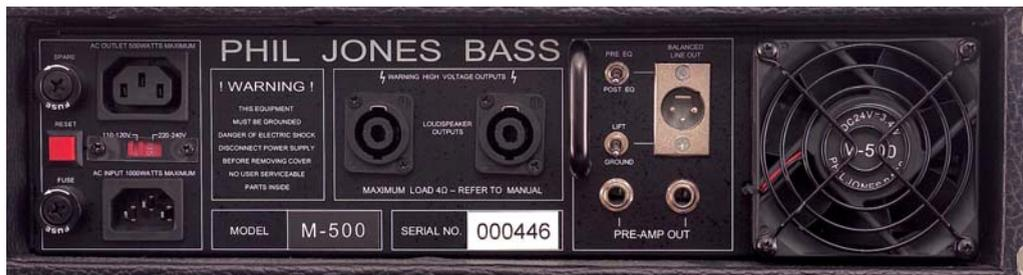
The M-500's rear panel includes an AC outlet, parallel pre-amp out jacks, and a full-featured balanced XLR output.
